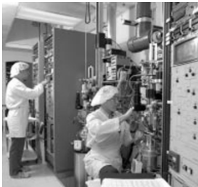
Fig. 8. Vertical dipping Hg-melt LPE growth systems employ vessels containing several kg of Hg saturated with Cd. In addition to the Cd, dopants are added to produce either n- or p-type HgCdTe epitaxial films.
