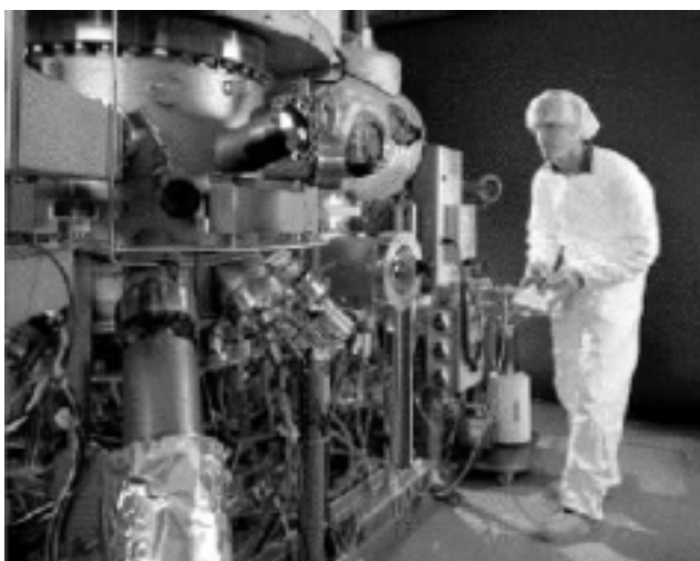
Fig. 9. HgCdTe MBE system. This system has a 5-inch (125 mm) susceptor to hold large substrates.
