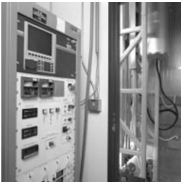
Fig. 5. Furnace and controller for growing CdZnTe boules.
